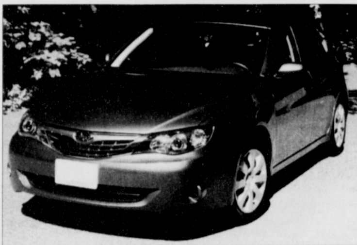
Specifications: 2.5-Liter 224-hp @ 226 lb-ft. torque Horizontally-Opposed SOHC Engine with Symmetrical AWD; 4-Speed Automatic w/Sportshift transmission; 20-City 27-Highway MPG; $20,303. MSRP
