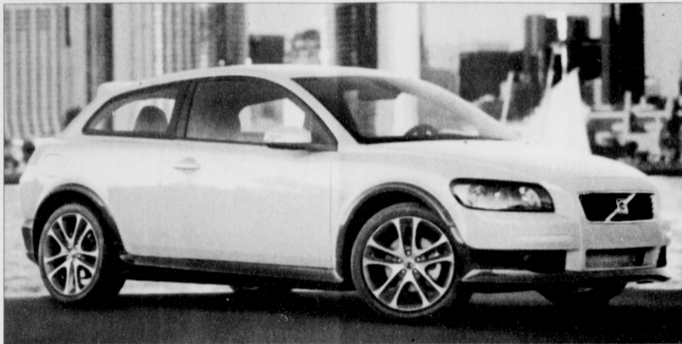
SPECIFICATIONS: 2.5-Liter, 5-Cylinder 227-hp @ 236 lb-ft. torque Turbocharged Engine; 6-Speed Manual transmission; 19-City 28-Highway MPG; $27,950. MSRP
