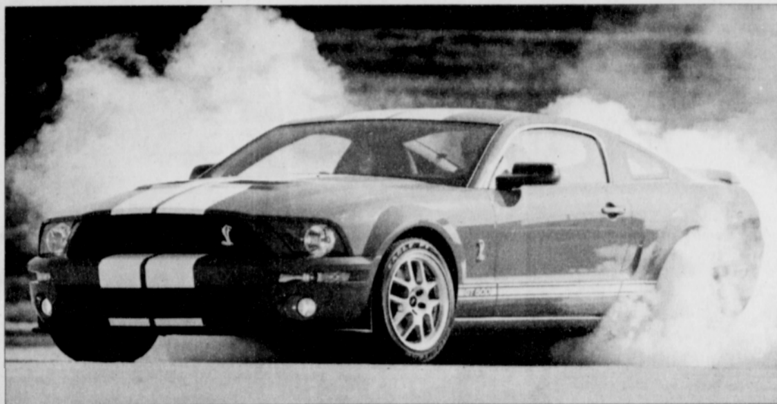
Specifications: 5.4-Liter, 500-hp@480 lb-ft. torque, V8, 32-Valve DOHC SMPI Engine; 6-speed manual transmission; 0-60 mph: 4.5 seconds; 15-City 21-Highway MPG; $43,765. MSRP
