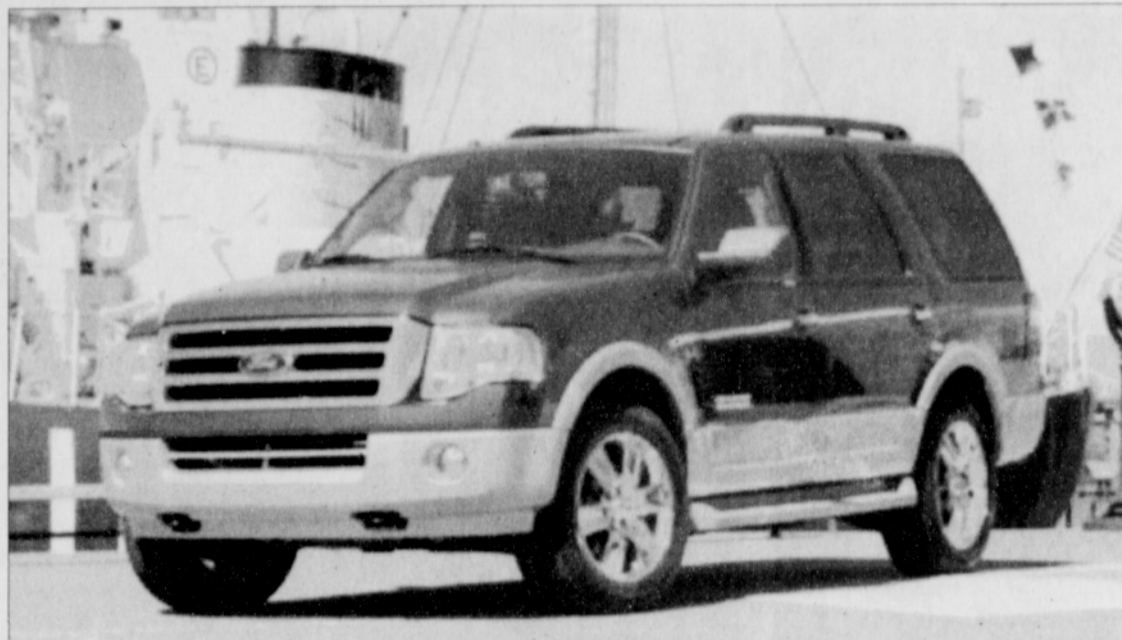
Specifications: 5.4-Liter 300-hp @ 365 lb-ft. torque, V-8 Engine; 6-Speed Automatic O/D Transmission; Electronically engaged 4-wheel drive; 14-City 20-Highway MPG; $47,610. MSRP
