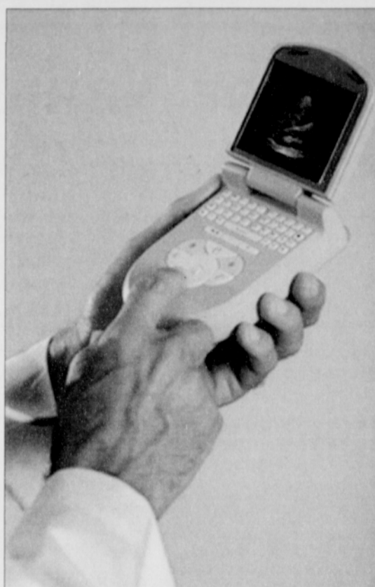
An ultrasound device for imaging the heart is starting to be used for taking images of arteries to determine risk of heart disease. (AP photo)
