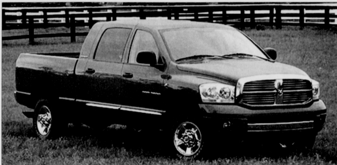
Specifications: 5.9-Liter I-6 325-hp Cummins Turbo-Diesel @610 lb-ft torque Engine; 4WD, 4-Speed Shift-on-the-Fly Automatic Transmission; 16-City 20-Highway Mpg; $54,395 MSRP.
