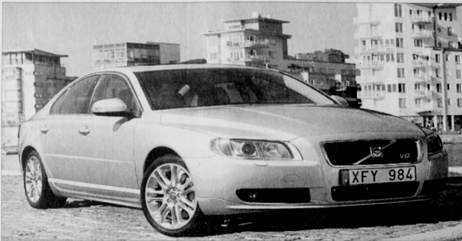
Specifications: 4.4-Liter, 8-Cylinder, 311-Hp @ 5950 RPM & 325 lbs.-ft. Torque @ 3950 RPM Engine; AWD, Geartronic 6-Speed Automatic Transmission w/Adaptive Shift Logic; 17-City 25-Highway MPG; $56,025 MSRP
