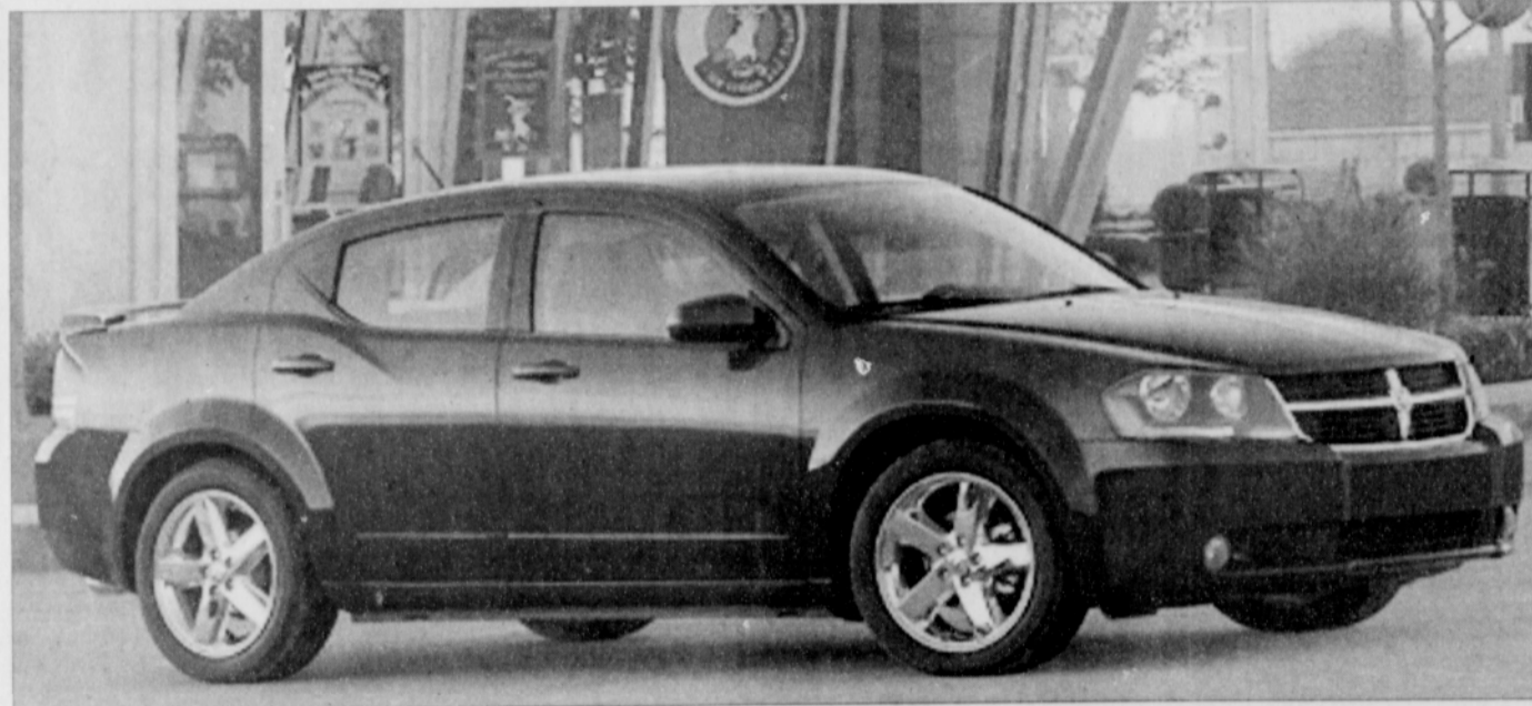
Specifications: 2.4-Liter 4-Cylinder World Engine 173-hp @ 166 lb-ft. torque, 4-Speed Automatic Transmission, 21-City mpg 30-Highway mpg, $19,125 MSRP
