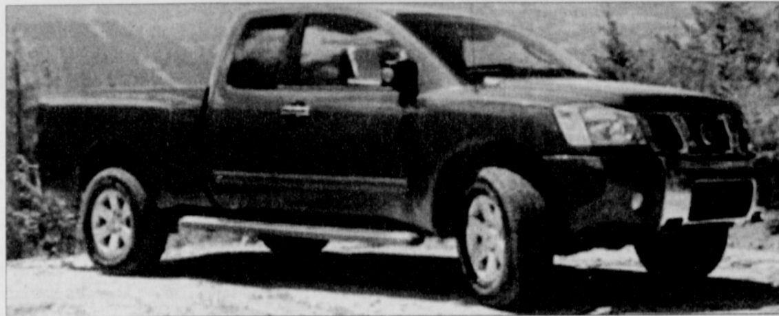
SPECIFICATIONS: 5.6-Liter, 32-Valve Endurance V-8 engine; 5-Speed Automatic transmission w/ Tow/Haul Mode; Shift-on-the-Fly 4WD System; 13-City mpg. 18-Highway mpg.; $38,255 MSRP
