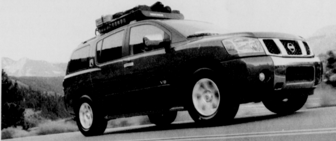
2006 Nissan Armada SE-OR 4X4 has 13 mpg city / 18 mpg hwy gas mileage; 5.6L V8, 32 valve, 305 hp @ 4900 rpm engine; 5 speed automatic transmission.
