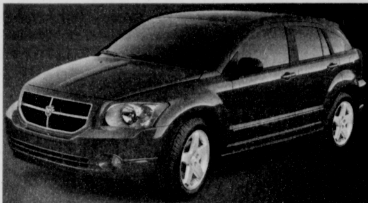
Tested Vehicle Information: Price: $21,300; Engine: 2.4 L multiport injection; Transmission: Continuously Variable Transaxle
