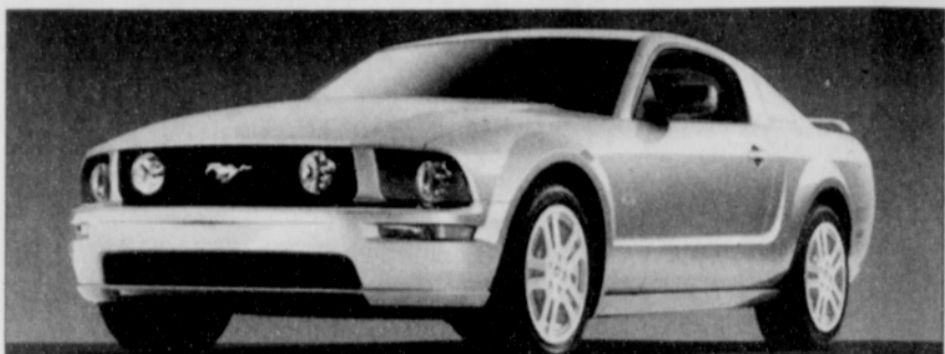
Tested Vehicle Information: Price: $27,630; Engine: 4.6 L 3V OHC V8; Transmission: 5-Speed Manual.
