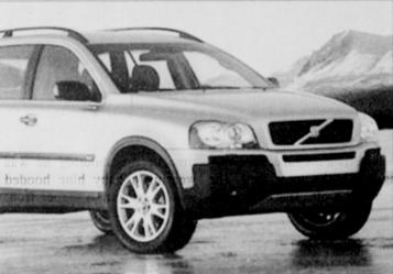
Tested Vehicle Information: Price: \$44,520; Engine: 2.5 liter intercooled light pressure turbo, 5 cylinder Alloy Engine; Transmission: Geartronic 5-speed automatic w/adaptive shift logic
