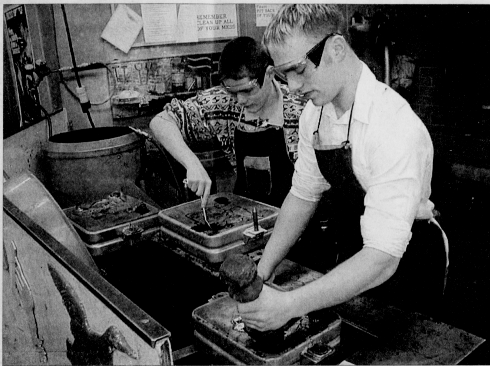
Metal shop students Ilya Grigoryev (left) and Randy Flowers of Franklin High School show off their award winning techniques to create sand molds for aluminum casting. Franklin recently won first and fifth place awards in a design and die-casting contest sponsored by the Northwest Chapter of the American Foundry Society.
