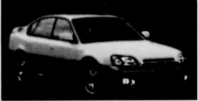
cle with 7.3 inches of ground clearance. The resulting high center of gravity makes the Outback Limited feel somewhat top heavy during quick maneuvers.
