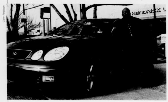
new twist with the GS400 V8: variable valve timing, the first ever used on a V8, according to Lexus, Toyota's luxury car division. You get a 300-horsepower boost in return and acceleration of zero to 60 in a mere six seconds. The GS400 has a top speed of 149 mph.
