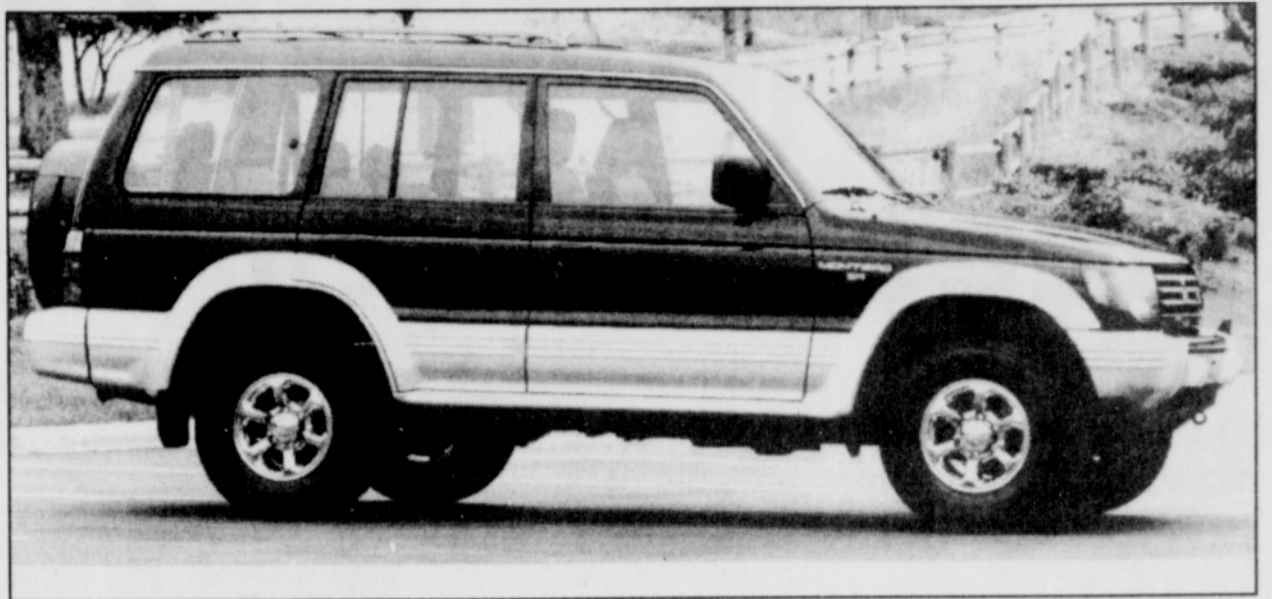
Mitsubishi Motor Sales Of America, Inc.: Thanks to its wide, aggressive stance, the '95 Montero SRis well suited for a variety of on- and off-road driving conditions. A 3.5 liter, double overhead -cam (DOHC), 24-valve V6 engine delivers 214 horsepower at 5,000 rpm and 228 ft.lbs. of torque at 3,000 rpm. For 1995, new features include: standard power sliding sunroof; optional adjustable shock absorbers (reintroduced for '95 as part of leather and wood package); a coded ignition key and a redesigned multi-meter combination comprised of oil pressure, compass, outside temperature and voltage gauges. Other standard equipment items include: a drivers-side air bag; Active Trac 4WD; ant-lock brakes; electronically controlled four speed transmission; and power windows and door locks.
