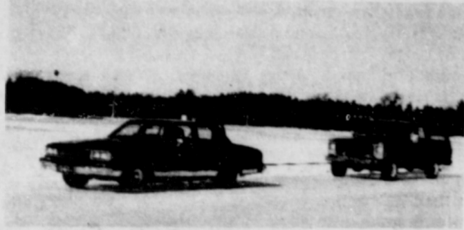
In the above scene at the National Safety Council's test project at Stevens Point, Wisconsin, pulling ability of the passenger car is being measured on a glare ice test course. The light truck is used as the "hold-back" vehicle and is connected to the test car using an instrumented drawbar that measures the pounds of pulling ability developed by the test car.
