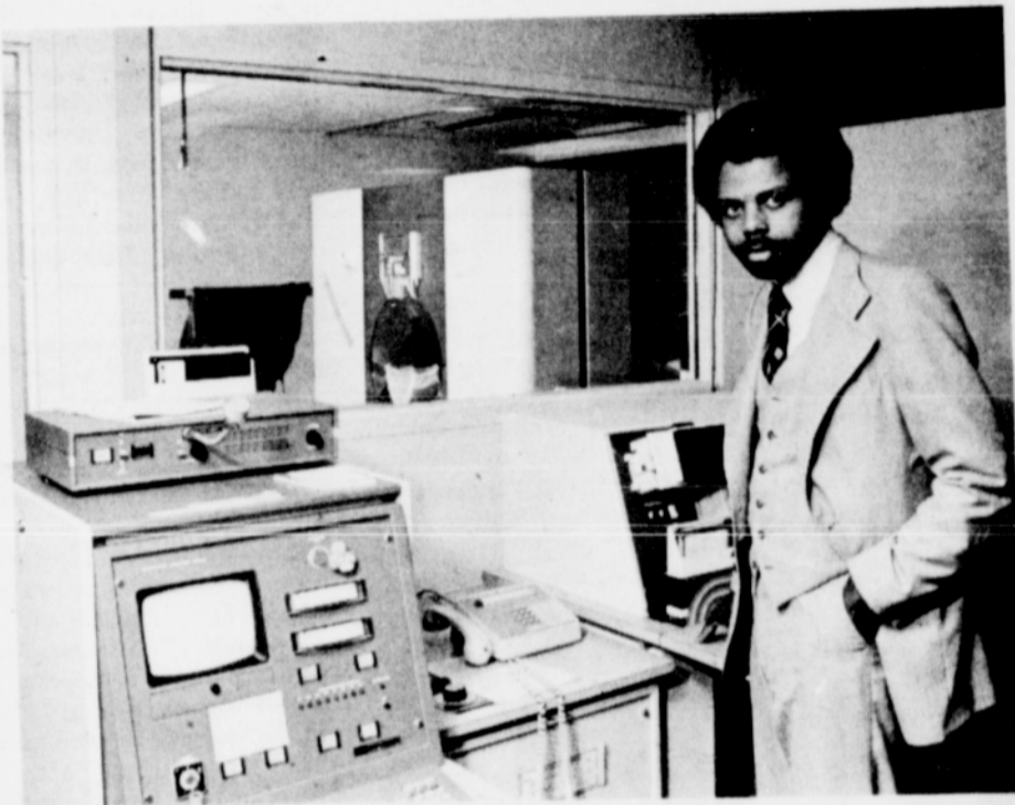
Ben Berry at CAT Scanner (Computed Axial Tomography) at Good Samaritan Hospital. Computer uses X-ray and sophisticated techniques to give cross-section views of the body's interior that can reveal organ damage, strokes and tumors.
