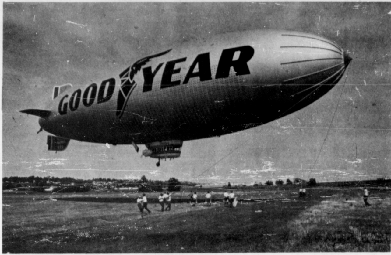
The Goodyear blimp, Columbia, comes in for a landing in Vancouver. The Columbia is 192 feet long, 59 feet high and 50 feet wide. The car, which is 23 feet long, carries six passengers and pilot. The ship is driven by twin Continental engines (6 cylinders, 210 hp each), with a maximum speed of 50 mph and a cruising speed of 35 mph. The envelope is made of rubber-coated polyester fabric.
