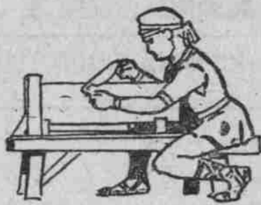
(1) Sawing mighty logs into bolts of stave length; splitting bolts into blocks to keep straight grain.
