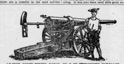
4.7-INCH QUICK-FIRING NAVAL GU N ON IMPROVISED CARRIAGE.
