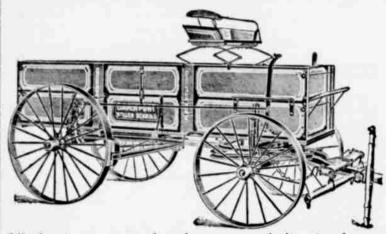
Oil about once a week, when wagon is in steady use, through automatically closing oil cups. Not necessary to remove wheels.
