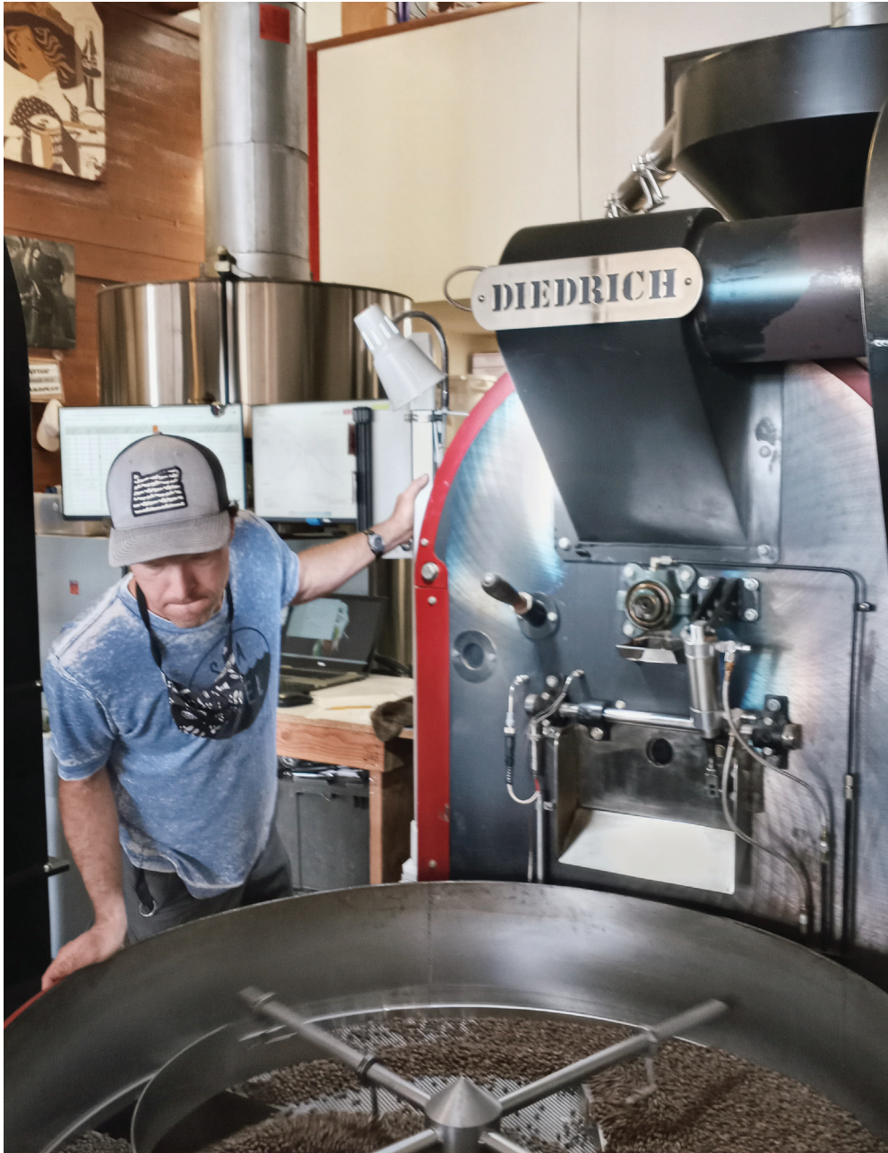
Photos by Gregory Zschomler ABOVE: Coffee beans cool in a cooling tray during one step of the roasting process. BELOW: Josh Olson, head roaster at Columbia River Coffee Roaster, watches a batch of beans as they rotate in the Diedrich roaster.
