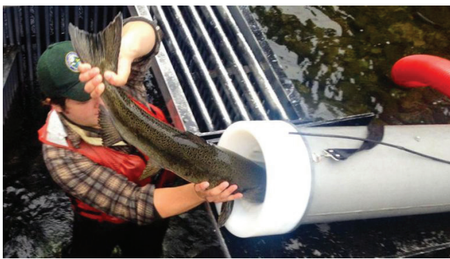
Courtney Flatt/Northwest News Network Washington Department of Fish and Wildlife crews load a 30-pound fall Chinook salmon into a demonstration of the original salmon cannon.
