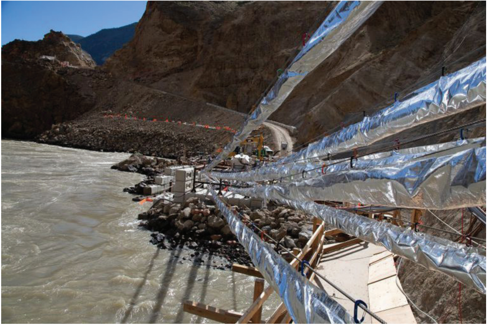
Whooshh Innovations A fish passage technology developed by Whooshh Innovations transported 8,200 salmon around a massive landslide on the Fraser River in a remote part of British Columbia.
