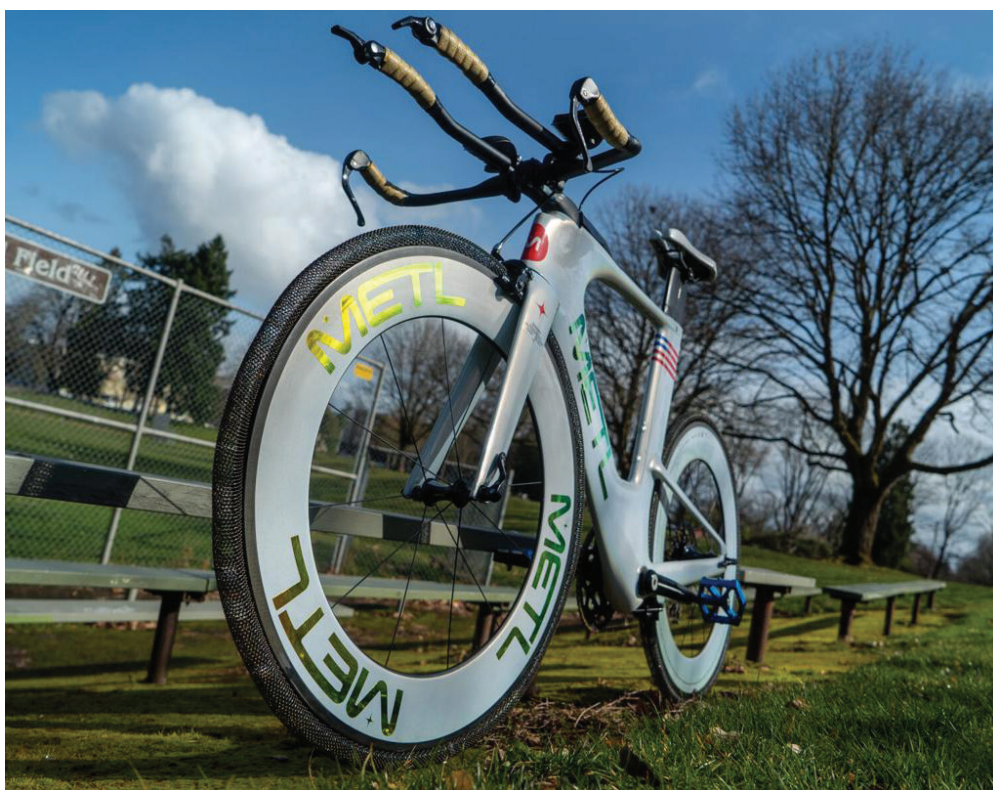
Bend native Calvin Young adapted the Mars rover tires into airless bicycle tires.
