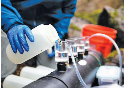
Penaluna pours river water into a filtering device to extract particles for environmental DNA analysis.
