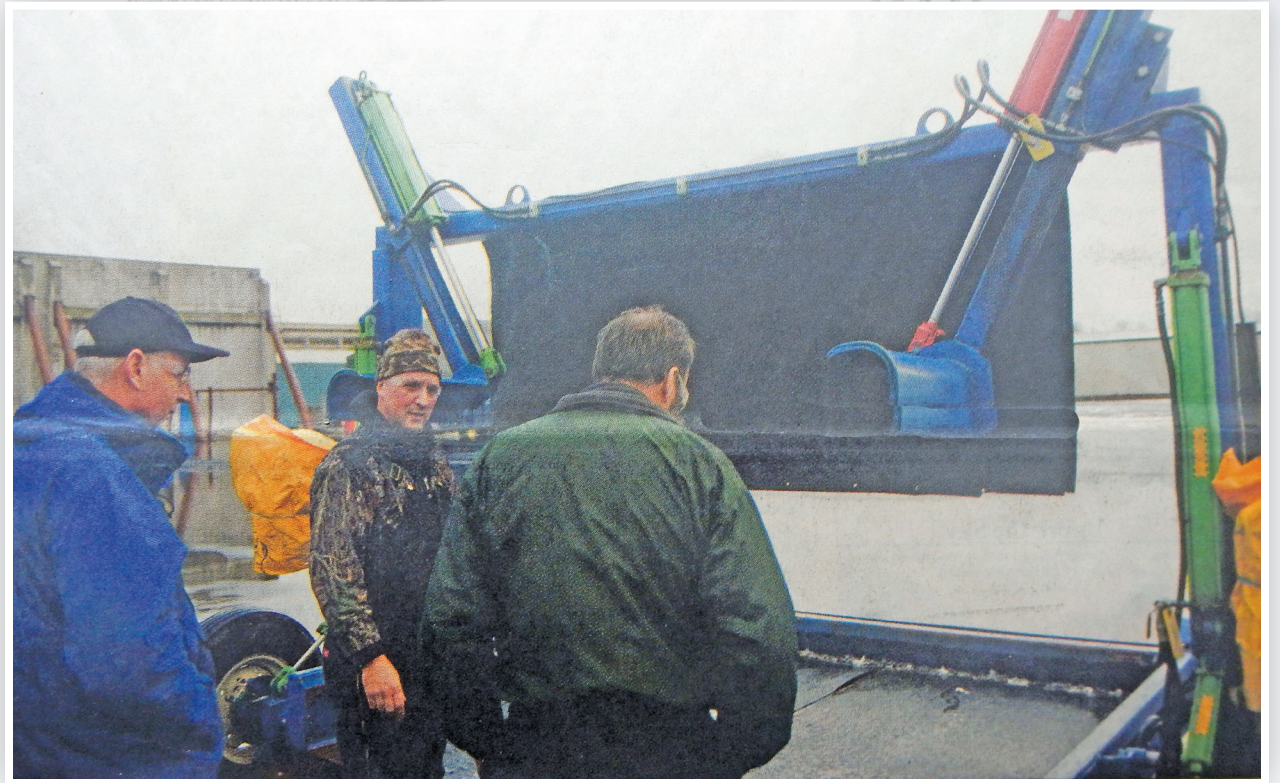
Scott Green, center, describes some of the modifications needed to turn the Ag-Bag Forage Solutions bale wrapper into a Flex-Tube Bagger, used to wrap stacks of pulp at Wauna Mill in 2011.
