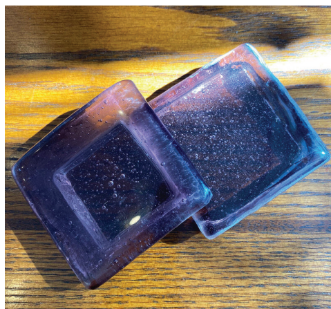
Photos by Lower Columbia Preservation Society TOP: A glass tile is removed before being replaced. ABOVE: New glass tiles made by Jamie Boyd. RIGHT: A restored vault light panel, outside Table 360 Bakery & Bistro.
