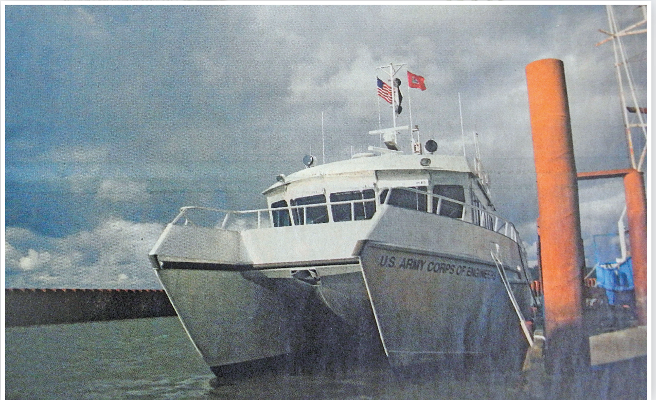
The U.S. Army Corps of Engineers' survey vessel Elton, stationed at Astoria's East Mooring Basin in 2010. It is designed to gather data on the river bottom of the Columbia River shipping channel using multibeam sonar technology.
