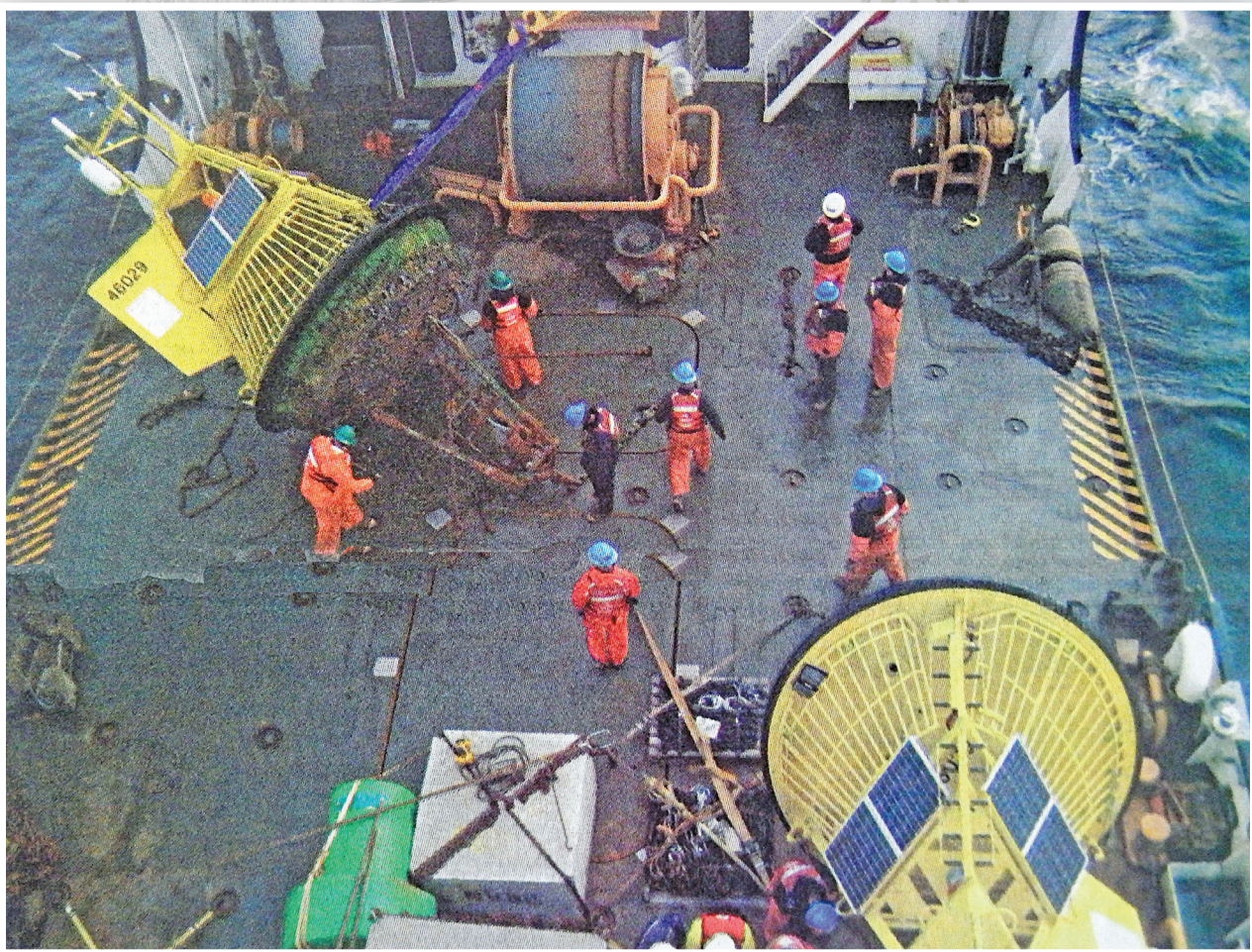
Two weather buoys, one recently retrieved, left, and one waiting to be installed, sit aboard the U.S. Coast Guard cutter Fir. The crew aboard the cutter hauled up an older buoy and replaced it with a newer model right before a storm.
