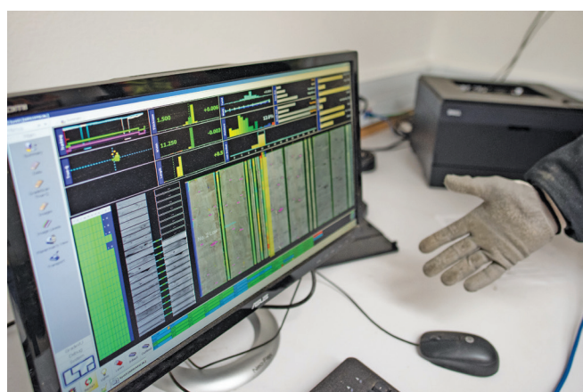
LEFT: Hampton Lumber mill workers use computers that help analyze lumber quality by taking photos of each piece as it passes through. RIGHT: Hampton Lumber CEO Steve Zika helped purchase the Warrenton mill in 2009 and has worked to fix and update the plant to increase production.
