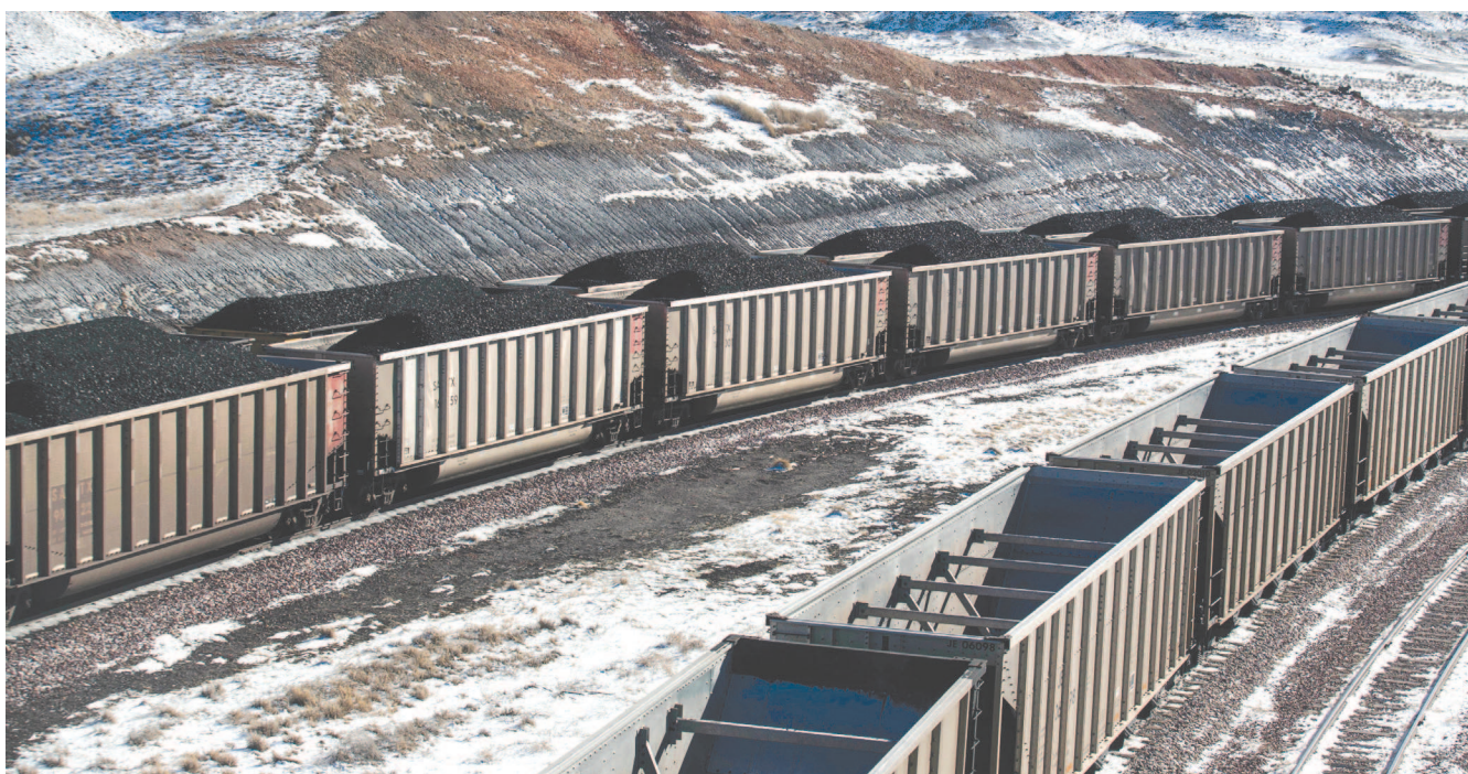
Rail cars are filled with coal and sprayed with a topper agent to suppress dust at Cloud Peak Energy's Antelope Mine north of Douglas, Wyo., in 2014.
