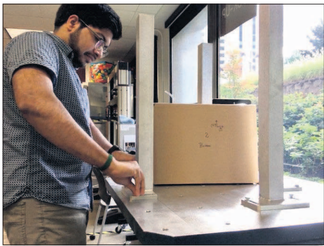
Cassandra Profita/Oregon Public Broadcasting BillerudKorsnäs designers use a shaking machine to test the protective power of the paper packaging they create.
