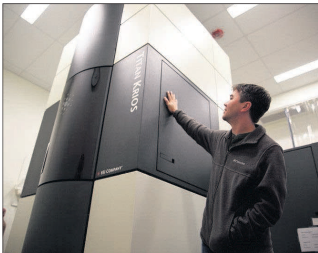
Kristian Foden-Vencil/Oregon Public Broadcasting A 2012 version of the four new cryo-electron microscopes that are coming to Oregon Health & Science University.
