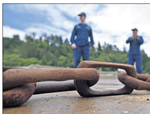
Chains up to an inch in diameter are commonly used to hold buoys in place.
