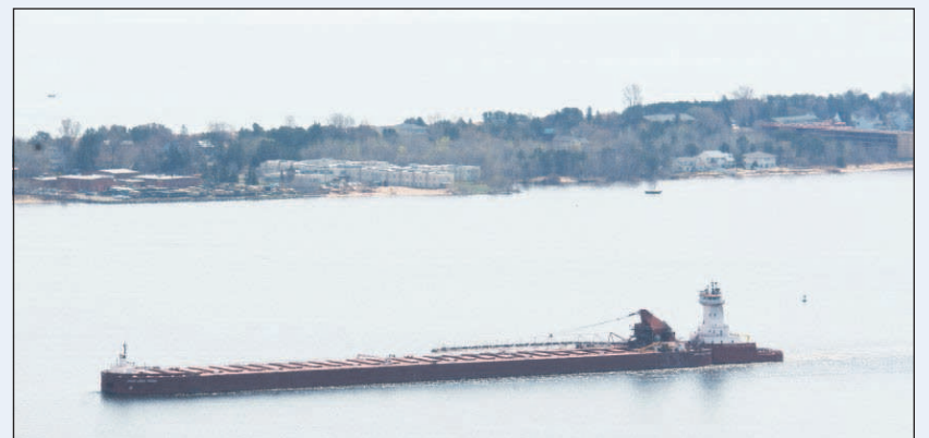
Wikimedia Commons About half of bulk oil-carrying vessels on the Columbia River were articulated tug barges. The barges include a notch in the bow, into which a tug hooks to propel and navigate.
