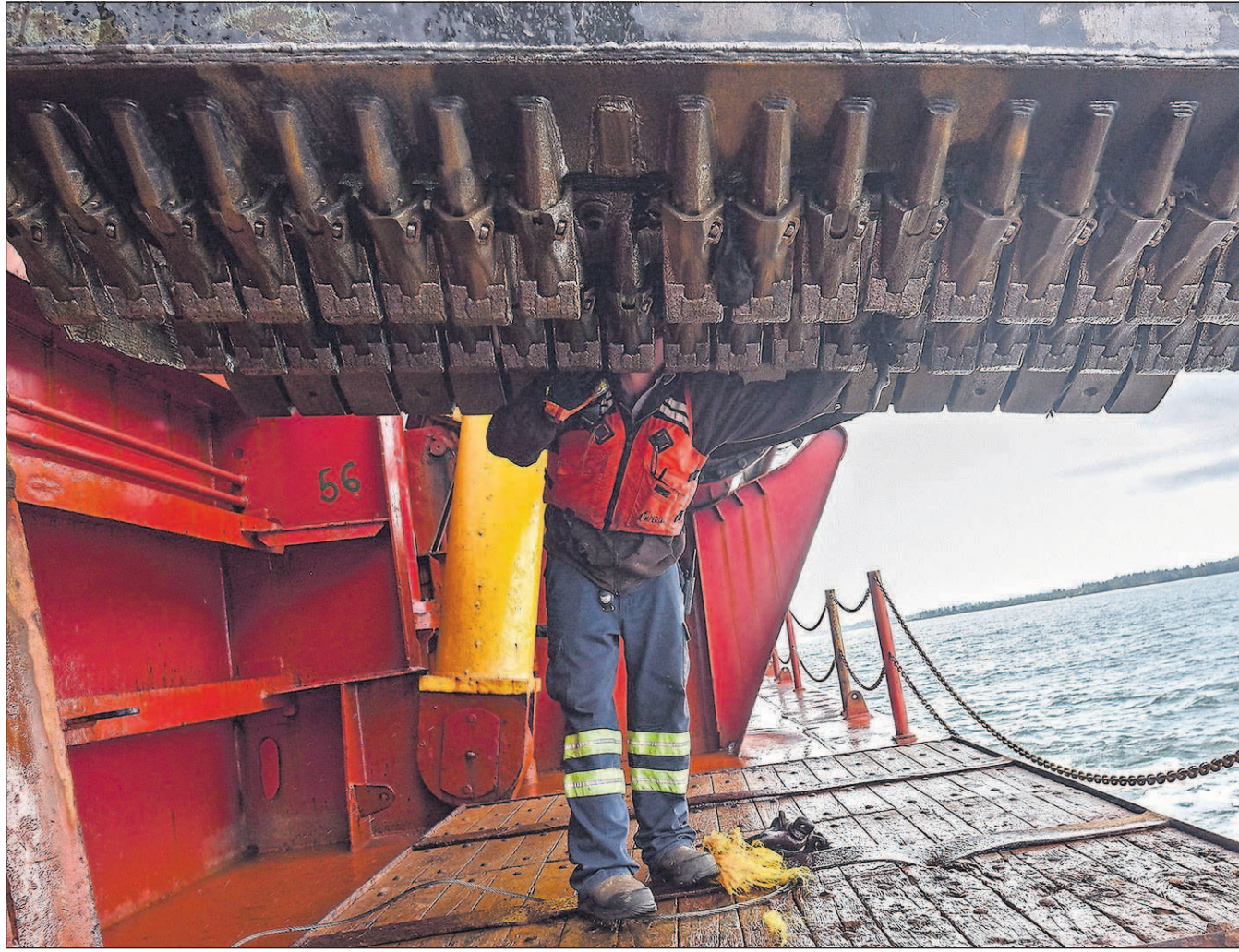
Photos by Colin Murphey/The Daily Astorian A crew member on the Terrapin Island dredging vessel inspects a section of the dredge arm that submerges below the surface of the Columbia River.
