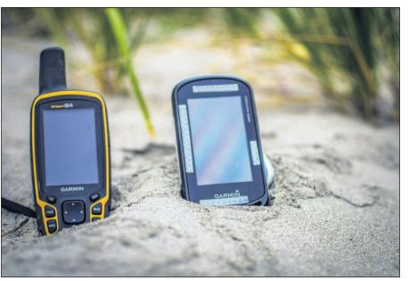
Two Garmin GPS units that Breniman carries — a touchscreen for fair-weather use, along with a unit with manual buttons for poor weather and search-andrescue applications.
