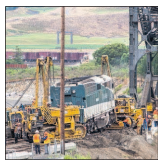
Peter Haley/The News Tribune Crews put a derailed Amtrak locomotive back on the tracks Monday in Steilacoom next to the bridge over Chambers Creek, Wash.
