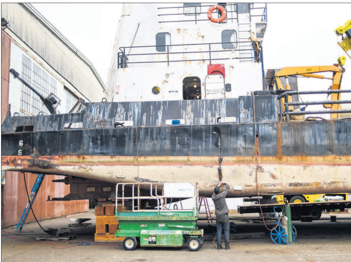
WCT Marine & Construction Inc. employee Jeremy Milligan works to cut the outerskin of a ship in order to remove an engine in 2016, at North Tongue Point in Astoria. The WCT and J&H Boatworks warehouses are adjacent to one another and the businesses sometimes work together on repair jobs.
