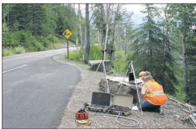
A National Park Service staffer sets up an acoustic recording station on Going-to-the-Sun Road to capture the impact of traffic on acoustic conditions in Glacier National Park, Mont. National Park Service
