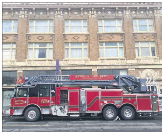
Erick Bengel/The Daily Astorian A 2016-model chassis from Pierce Manufacturing, the Astoria Fire Department's new ladder truck has a 105-foot ladder and a dual-rear axle.
