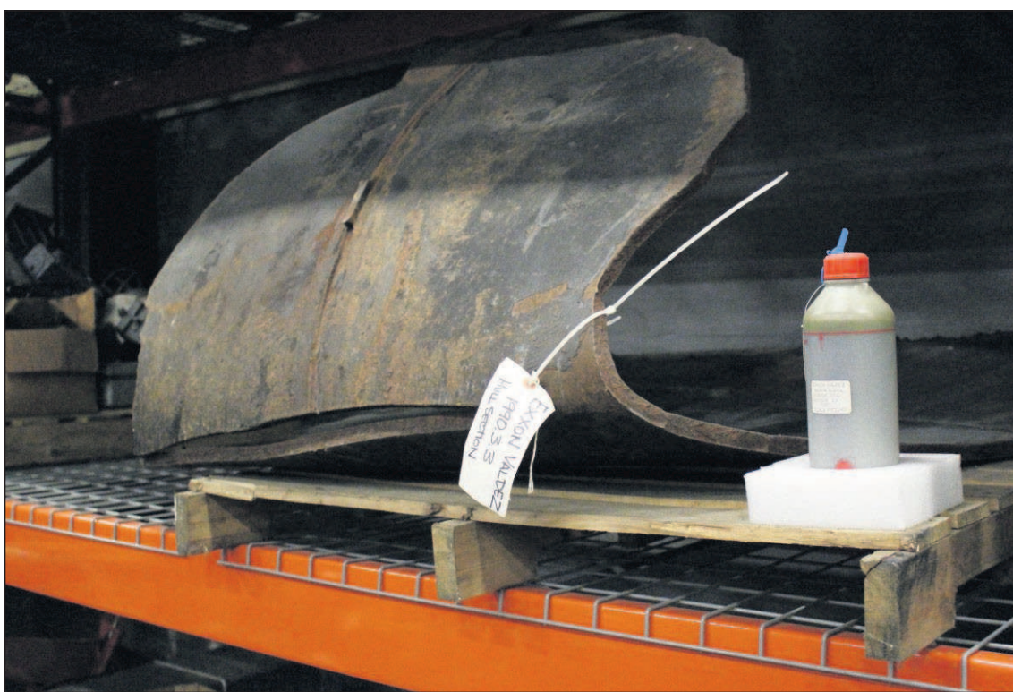
The fractured piece of hull plating from the Exxon Valdez — the part of the tanker that broke on the Bligh Reef and spilled gallons of oil in Alaskan waters — resides in the Columbia River Maritime Museum's collections storage facility. On the right is a bottle of the oil.
