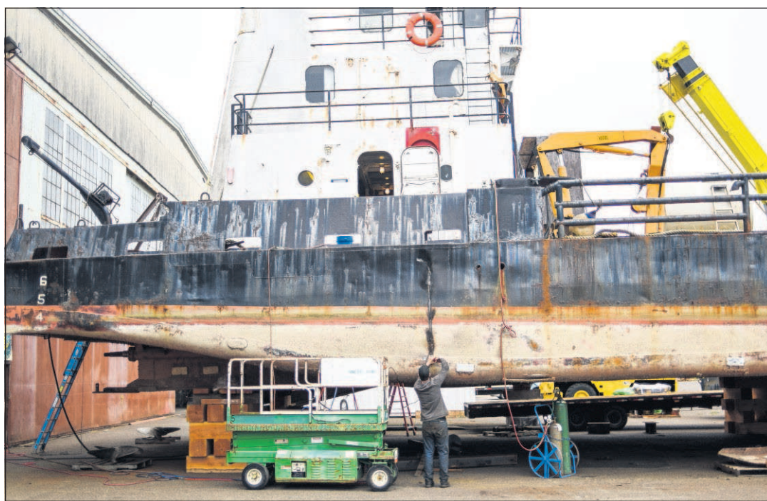
WCT Marine & Construction Inc. employee Jeremy Milligan works to cut out the outer-skin of a ship in order to remove an engine. The WCT and J&H Boatworks warehouses are adjacent to one another and the businesses sometimes work together on repair jobs.
