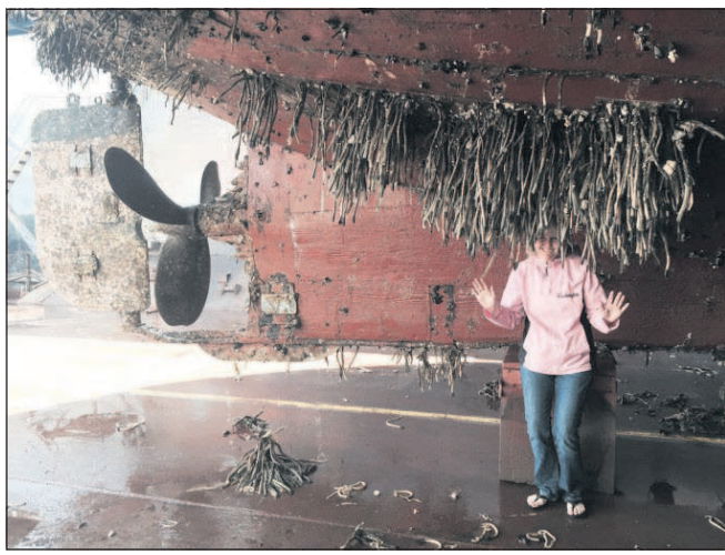
Photo courtesy of Christian Lint Melissa Lynch, marketing director for the Tourist No. 2, aka MV Kirkland in Bremerton, Wash., stands beneath five years of tube worm growth on the bottom of the ferry, which is getting pressure-washed at Northlake Shipyard in Seattle this week.
