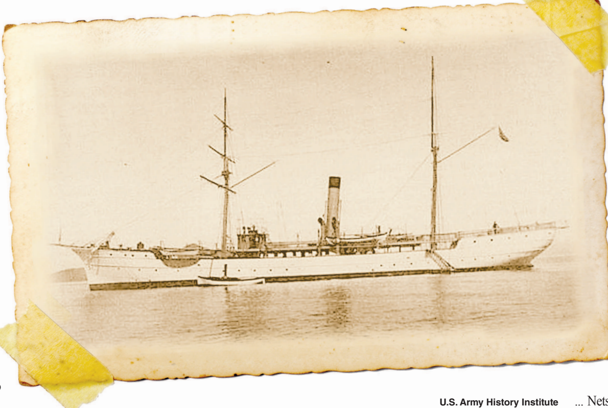
The USS Albatross was an iron-hulled, twin-screw U.S. Navy steamer. It may have been the first vessel ever built specifically for marine research, often operating out of the still-famous oceanographic science center at Woods Hole, Massachusetts. In 1887-89, the Albatross made a major survey of West Coast fisheries.
