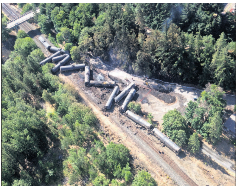
Washington Department of Ecology Scattered and burned oil tank cars are pictured, Saturday, after a train derailed and burned near Mosier, Friday. Union Pacific Railroad says it had recently inspected the section of track near Mosier, about 70 miles east of Portland, and had been inspected at least six times since March 21.
