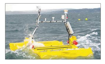
Startup Columbia Power (http://columbiapwr.com) has a new gizmo, StingRAY, which harnesses ocean waves and generates electricity, according to a story on CNN (http://tinyurl. com/stingwave). One is pictured, courtesy of Columbia Power.
