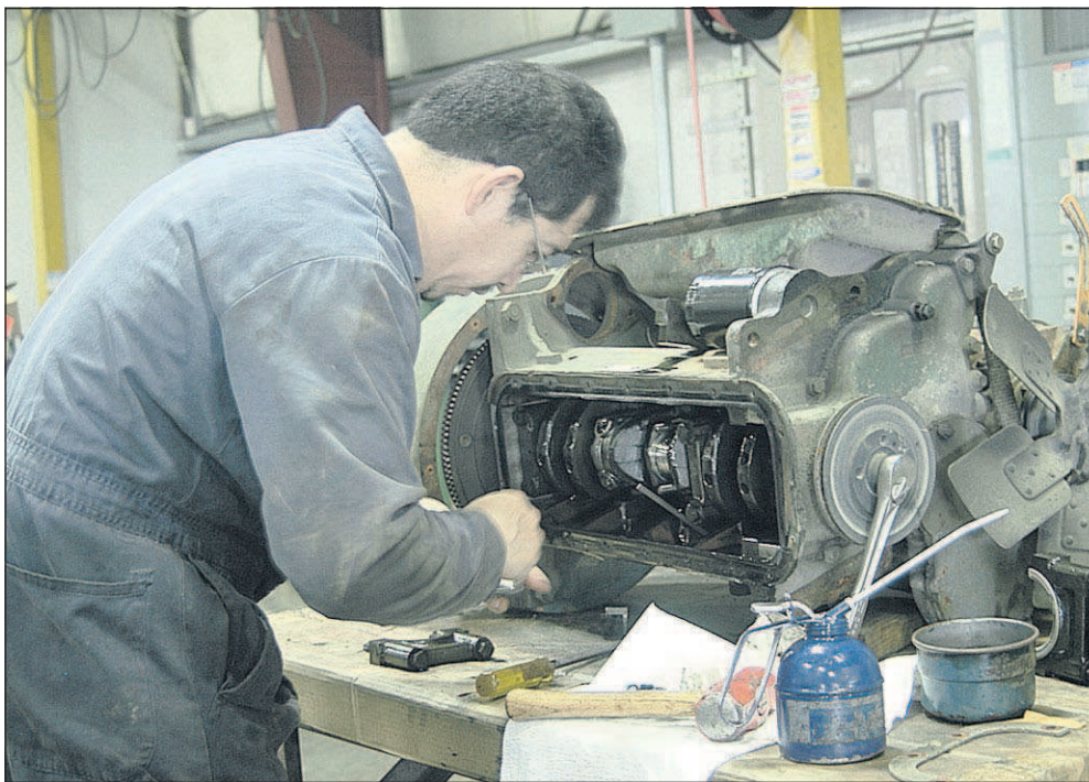
Jaime Perez, mechanic at Farmland Tractor Supply, rebuilds a Case engine for resale. The company, in business since 1980, often sells to beginning or small farmers who can't afford new equipment.
